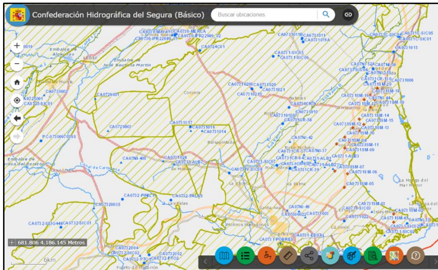
Figure 9: CHS web viewer with visible shapefiles of groundwater body boundaries (polygons) and quality network points.
